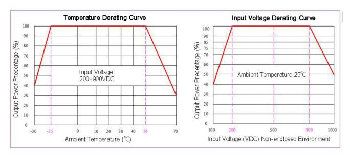
Note 1: When the input voltage is 100~1000VDC and the temperature is -30~70℃, voltage derating is required based on the input voltage derating curve.
