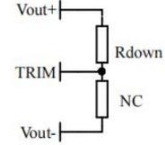
Voltage Down: Add resistor  $R_{down}$  between Trim and output positive
