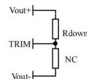
Voltage up regulation: add resistor Rup between Trim and output negative      Voltage Down: Add resistor Rdown between Trim and output positive
