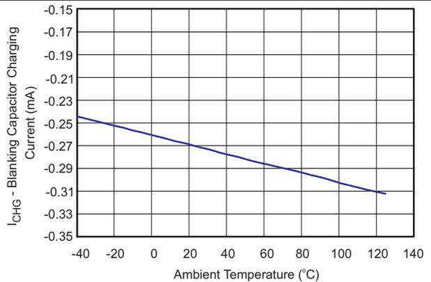
Figure 14. Blanking Capacitor Charging Current vs. Temperature
