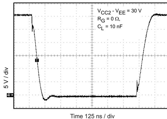
Figure 73. Output Waveform
