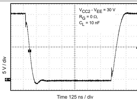
Figure 26. Output Waveform
