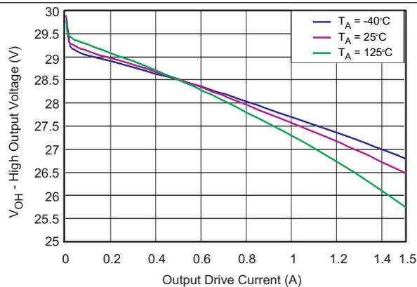
Figure 11. High Output Voltage vs. Output Drive Current
