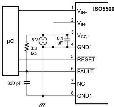
**Figure 63. FAULT Pin Circuitry for High CMTI**
