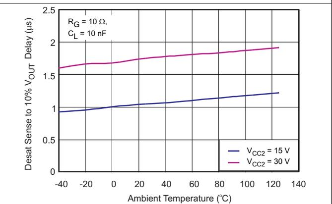
Figure 22. DESAT Sense to 10%  $V_{OUT}$  Delay vs Temperature
