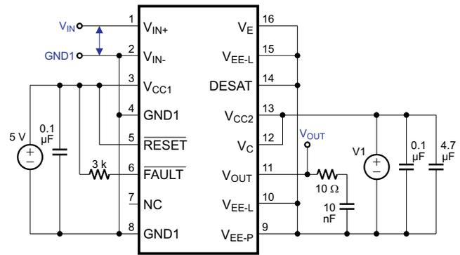
Figure 47.  $t_{PLH}$ ,  $t_{PHL}$ ,  $t_r$ ,  $t_f$  Test Circuit
