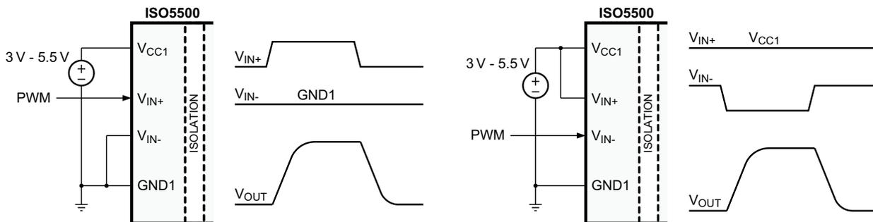
Figure 56. Non-inverting (left) and Inverting (right) Input Configurations
