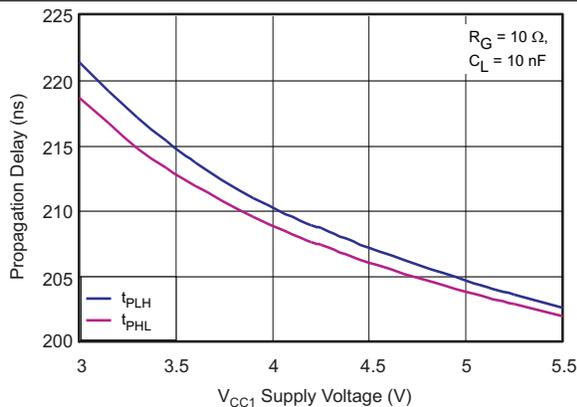
Figure 17. Propagation Delay vs. V<sub>CC1</sub> Supply Voltage
