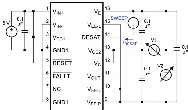
Figure 42.  $I_{CHG}$ ,  $I_{DSCHG}$ ,  $V_{DSTH}$  Test Circuit
