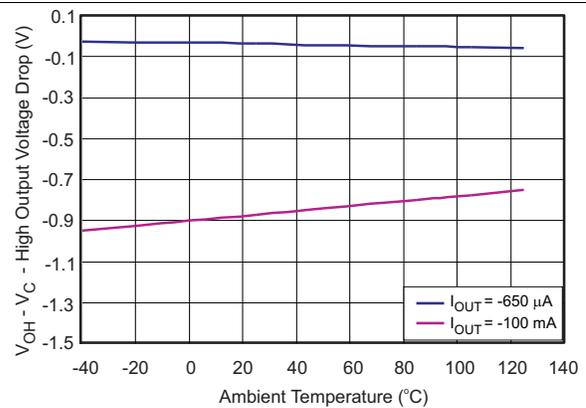
Figure 10. High Output Voltage Drop vs. Temperature
