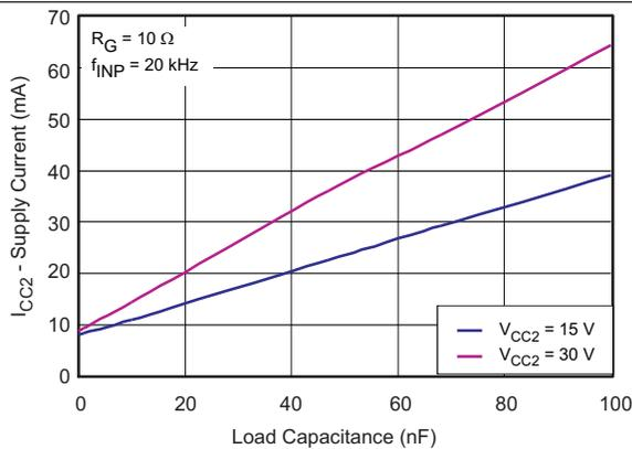
Figure 5.  $V_{CC2}$  Supply Current vs. Load Capacitance
