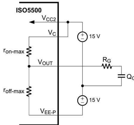
Figure 69. Simplified Output Model for Calculating P<sub>OL-wc</sub>
