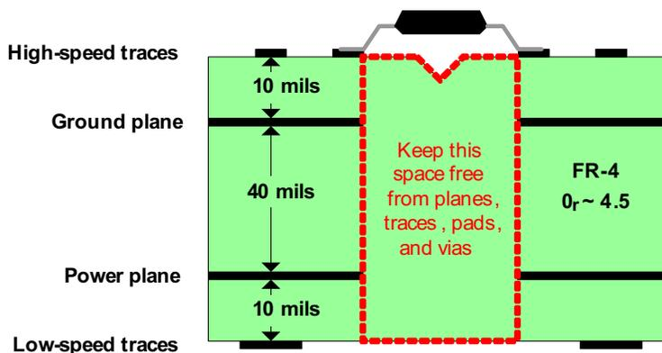
Figure 74. Recommended Layer Stack
