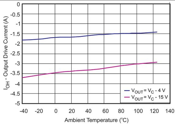
Figure 7. Output Drive Current vs. Temperature
