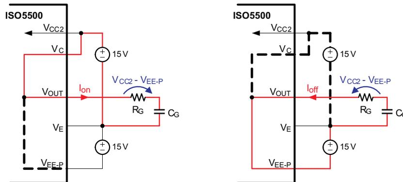
Figure 70. Simplified Gate Charge and Discharge Model
