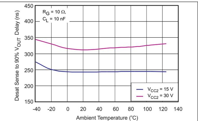
Figure 20. DESAT Sense to 90%  $V_{OUT}$  Delay vs Temperature
