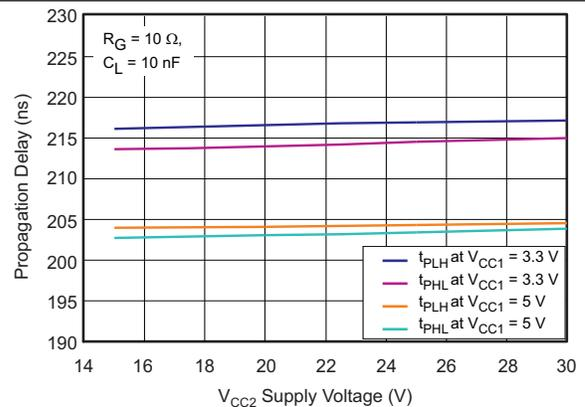
Figure 18. Propagation Delay vs. V<sub>CC2</sub> Supply Voltage
