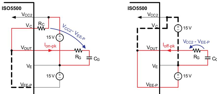
Figure 71. Reducing  $I_{ON-PK}$  by Inserting Resistor  $R_C$
