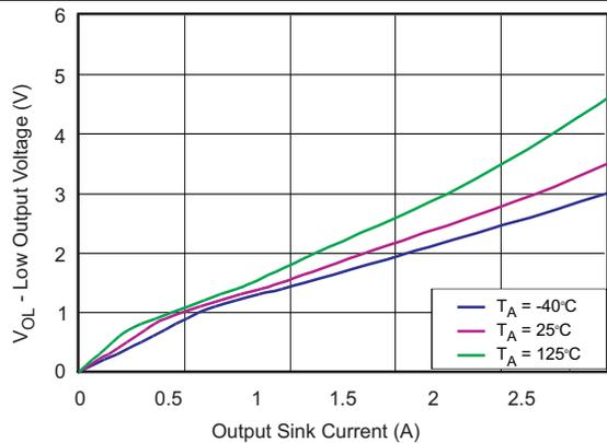
Figure 13. Low Output Voltage vs. Output Sink Current
