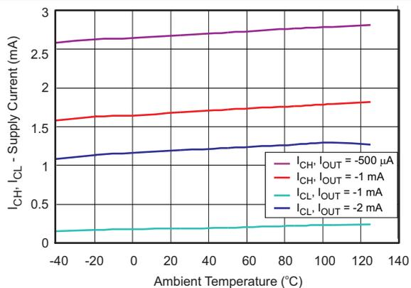
Figure 27. V<sub>C</sub> Supply Current vs. Temperature
