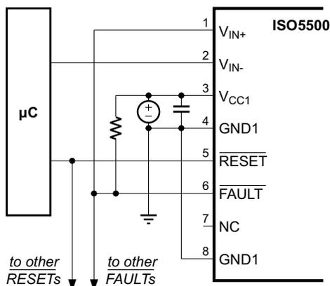
Figure 65. Global Shutdown with Inverting Input Configuration
