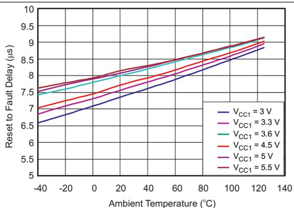
Figure 25. Reset to Fault Delay vs Temperature
