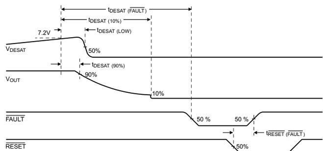
Figure 51.  $DESAT$ ,  $V_{OUT}$ ,  $FAULT$ ,  $RESET$  Delays
