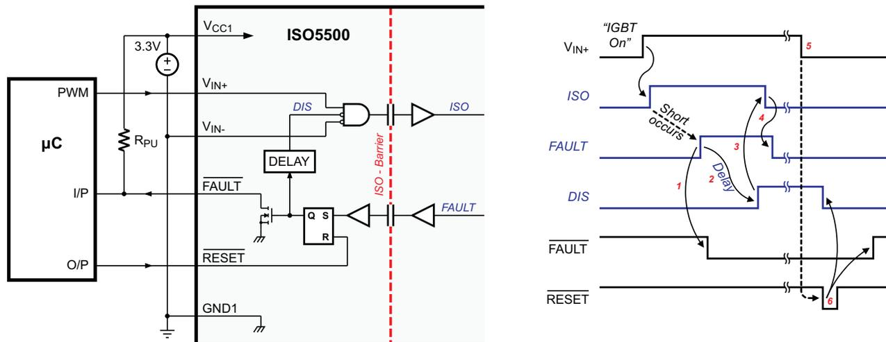
**Figure 60. Fault Alarm Circuitry and Timing Sequence**
